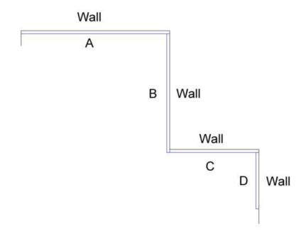
If you wish to use corner trims, this will give you a little extra tolerance in the lengths you need to measure. When using the trims, you can deduct an extra 2mm for each trim from a length. This means you can set the upstands with a little space between them and cover these gaps with the trim. So, in the example above you should deduct an additional 2mm from lengths **A** and **D**, and 4mm from **B** and **C**.
